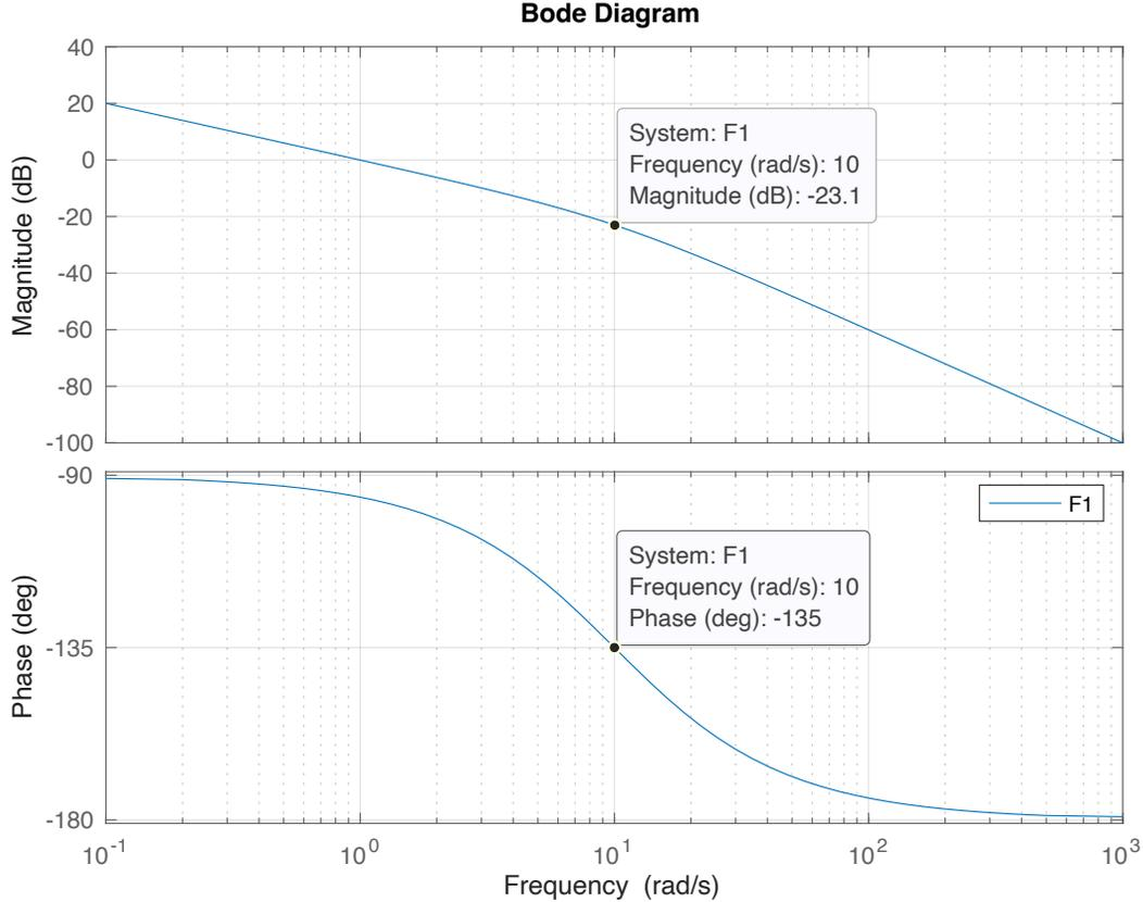
Therefore, we require a magnitude amplification of about 20 dB for  $F_1$  to have a crossing frequency  $\omega_c \cong 10$  rad/sec and a phase increase  $> 15^\circ$  to have  $\varphi_m > 60^\circ$  ( $\varphi_m = \pi - |\arg(F(j10))|$ ).
