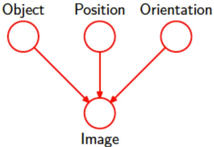
A graphical model representing the process (causal process) by which images of objects are created. The image (a vector of pixel intensities) has a probability distribution that is dependent on the identity of the object as well as on its position and orientation.
