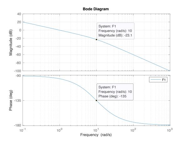
Therefore, we require a magnitude amplification of about 20 dB for  $F_1$  to have a crossing frequency  $\omega_c \cong 10$  rad/sec and a phase increase > 15° to have  $\varphi_m > 60° (\varphi_m = \pi - |\arg(F(j10))|)$ .
