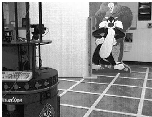
Figure 6.19 A Denning mobile robot using a color histogram to play tag with a poster of Sylvester and Tweety.
