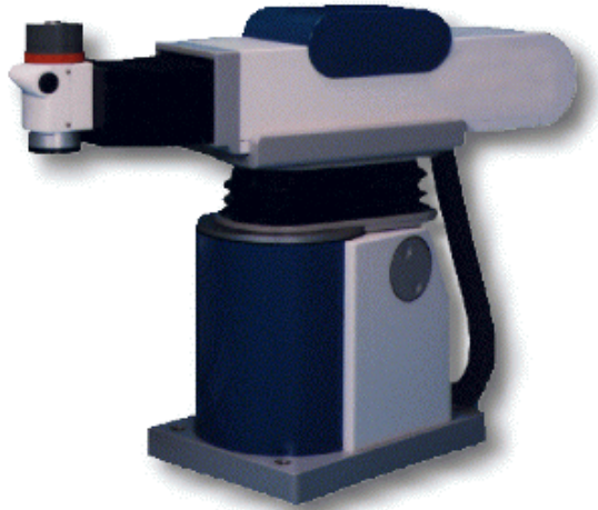
Figure 1.3 An RT3300 industrial manipulator. (Photograph courtesy of Seiko Instruments.)
