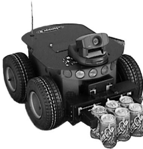
Figure 5.10 A Pioneer P2-AT with a forklift arm suitable for picking up soda cans. (Photograph courtesy of ActivMedia, Incorporated.)
