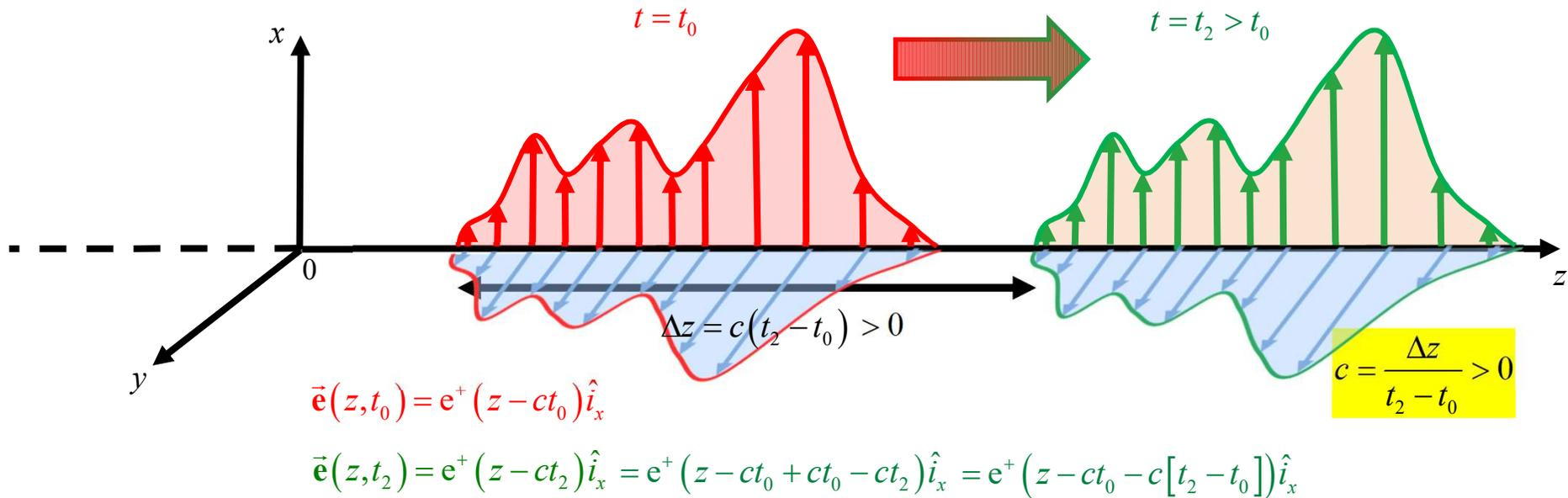
The electromagnetic perturbation **propagates** without deformation and with constant speed  $c$  along the positive sense of the  $z$ -axis
