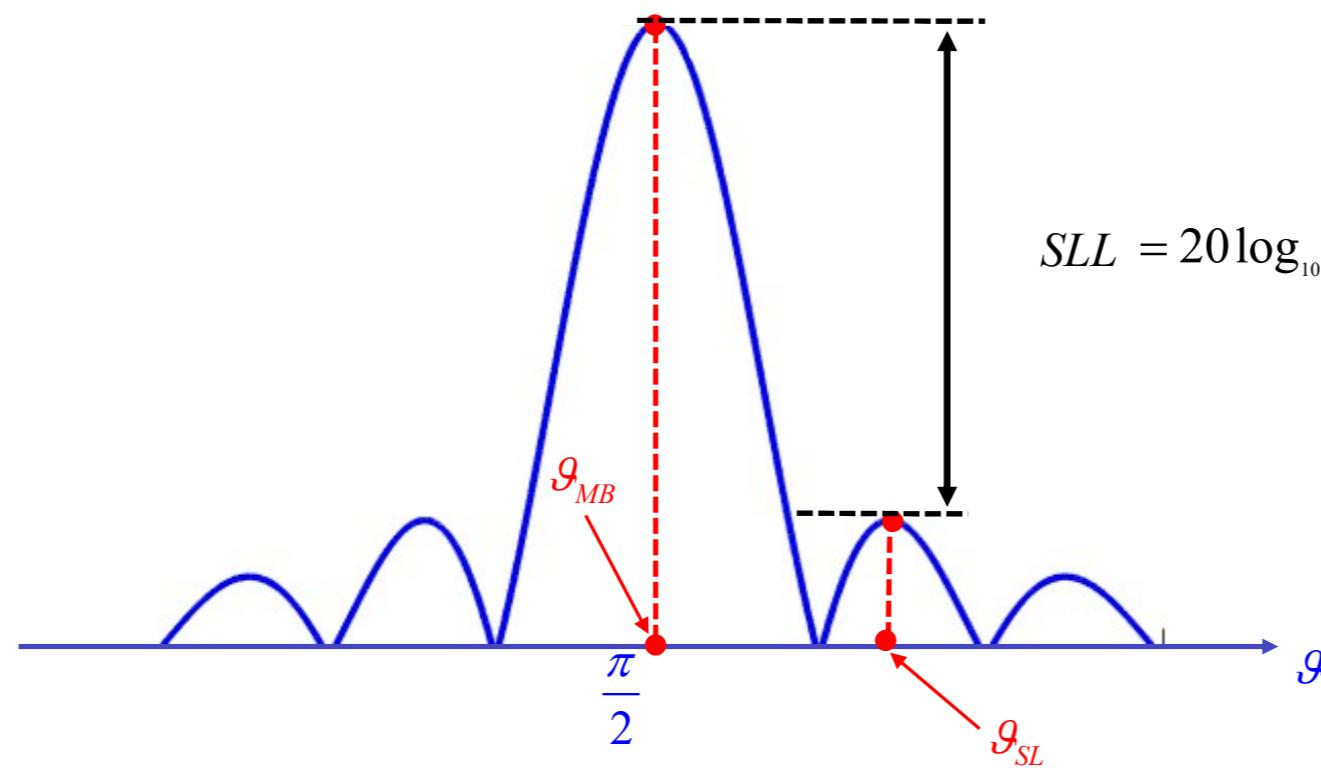
$$SLL = 20 \log_{10} \frac{|\vec{I}(\vartheta_{SL}, \varphi_{SL}) F(\vartheta_{SL})|}{|\vec{I}(\vartheta_{MB}, \varphi_{MB}) F(\vartheta_{MB})|} = 20 \log_{10} \frac{|F(\vartheta_{SL})|}{|F(\vartheta_{MB})|}$$
