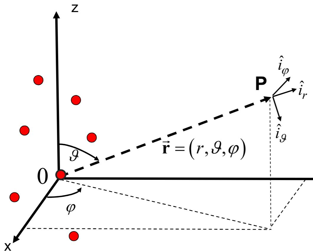
Let us suppose that P is located in the **Fraunhofer Region** relevant to the each antenna of the considered array
