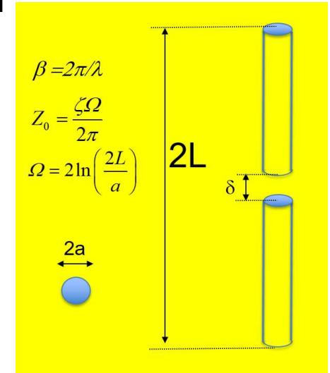
The Hallen model provides a wrong value of the input resistance  $R_{\text{in}}$ , due to the employed approximations. Actually, measurements carried out in laboratory show that, in contrast to the Hallen formulation,  $R_{\text{in}} \neq 0$ .
