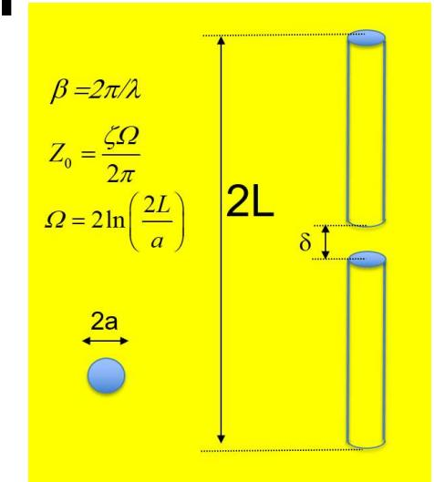
The Hallen model provides a wrong value of the input resistance  $R_{\text{in}}$ , due to the employed approximations
