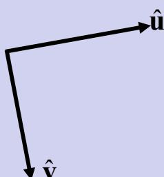
The vector  $\vec{f}(t)$  lies in the polarization plane ( $\hat{\mathbf{u}}, \hat{\mathbf{v}}$ ) and it changes in general both its amplitude and its direction as the time elapses.
