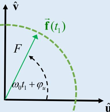
$$(|F_u| = |F_v| = F) \quad \text{and} \quad \left( \varphi_v - \varphi_u = \frac{\pi}{2} \right)$$
