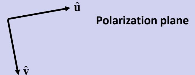
**Linear polarization:** the vector  $\vec{f}(t)$  does not change its direction and its tip moves along a straight line.
