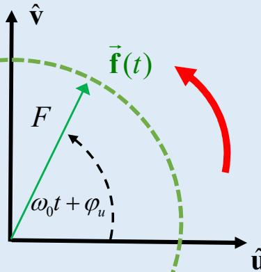
The vector  $\vec{f}(t)$  maintains a constant modulus and its tip moves along a circle with angular velocity  $\omega_0$
