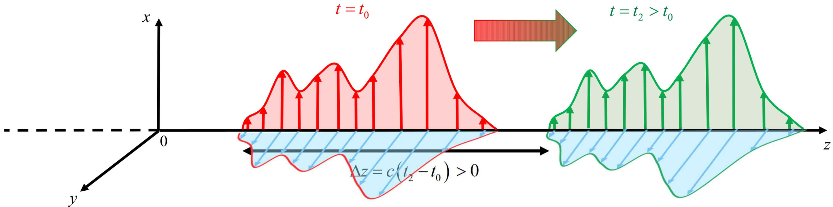
The electromagnetic perturbation **propagates** without deformation and with constant speed  $c$  along the positive sense of the  $z$ -axis
