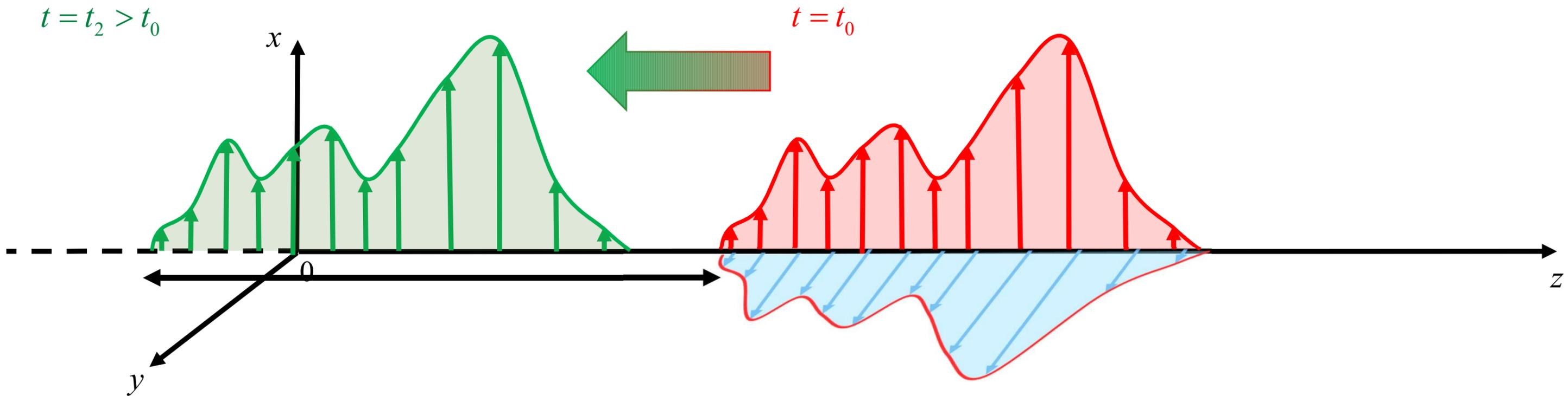
The electromagnetic perturbation **propagates** without deformation and with constant speed  $c$  along the negative sense of the z-axis
