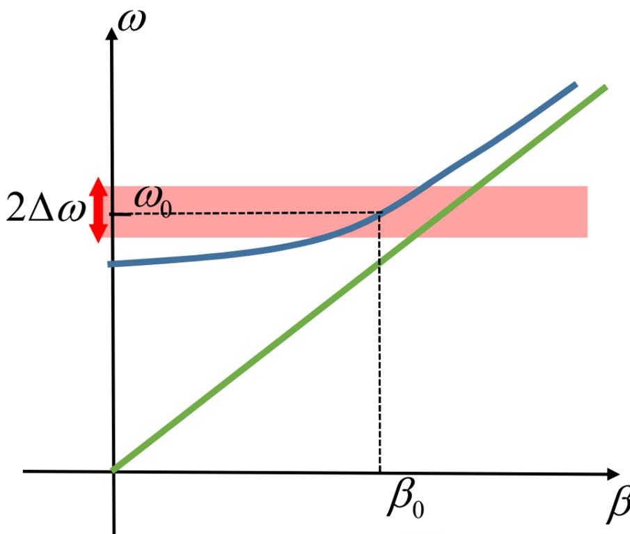
$$\beta(\omega) \approx \beta(\omega_0) + \beta'(\omega_0)(\omega - \omega_0) + \frac{1}{2}\beta''(\omega_0)(\omega - \omega_0)^2 + \dots$$
