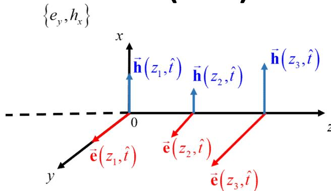
$$\begin{cases} \frac{\partial e_x}{\partial z} = -\mu \frac{\partial h_y}{\partial t} \\ \frac{\partial h_y}{\partial z} = -\epsilon \frac{\partial e_x}{\partial t} \end{cases}$$
