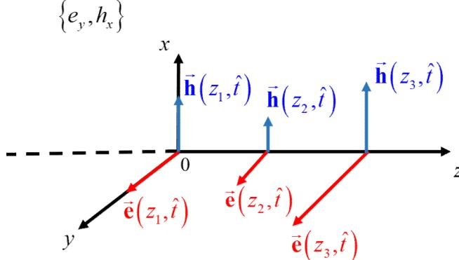
$$\begin{cases} \frac{\partial e_x}{\partial z} = -\mu \frac{\partial h_y}{\partial t} \\ \frac{\partial h_y}{\partial z} = -\epsilon \frac{\partial e_x}{\partial t} \end{cases} \quad \frac{\partial^2 e_x}{\partial z^2} = \mu\epsilon \frac{\partial^2 e_x}{\partial t^2}$$
