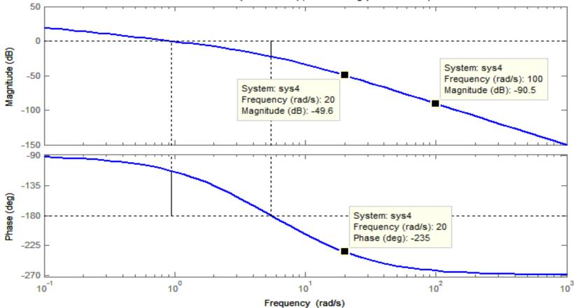
$\checkmark$  F'(s) magnitude amplification of  $50_{db}$  to have a crossing frequency  $\omega_c = 20$  rad/s
