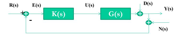
$$\begin{pmatrix} Y(s) \\ E(s) \\ U(s) \end{pmatrix} = \begin{pmatrix} \mathbf{T}(s) & \mathbf{S}(s) & -\mathbf{T}(s) \\ \mathbf{S}(s) & -\mathbf{S}(s) & -\mathbf{S}(s) \\ \mathbf{Q}(s) & -\mathbf{Q}(s) & -\mathbf{Q}(s) \end{pmatrix} \begin{pmatrix} R(s) \\ D(s) \\ N(s) \end{pmatrix}$$
