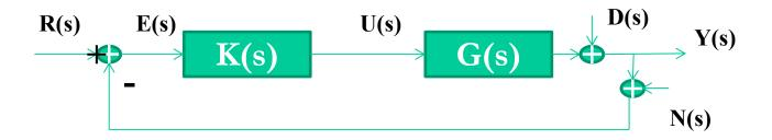
△ The dynamic relations between inputs and outputs of the systems are expressed by 9 transfer functions.
