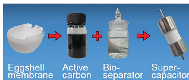
Fig. 25 Fabrication of an asymmetric supercapacitor using biowaste-derived materials from chicken egg shells. Adapted from ref. 258. Copyright 2018, with permission from ACS.
