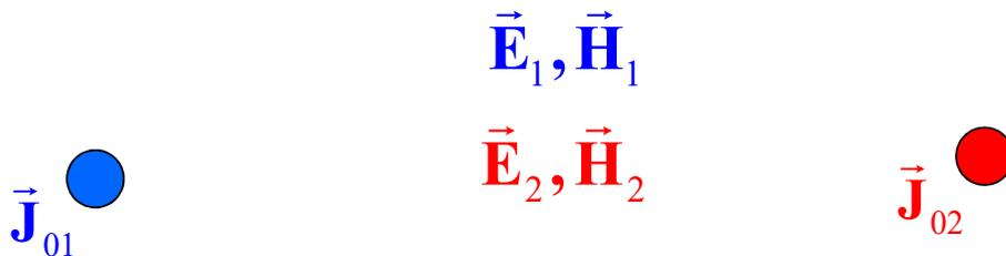
Consider a source distribution  $\vec{J}_{01}$  with its associated electromagnetic field  $(\vec{E}_1, \vec{H}_1)$
