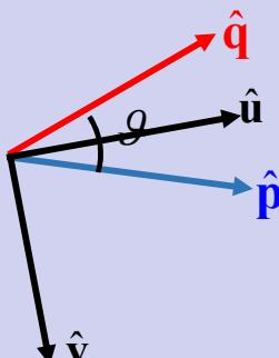
The vector  $\vec{f}(t)$  lies in the polarization plane  $(\hat{\mathbf{p}}, \hat{\mathbf{q}})$  (which is coincident with the plane  $(\hat{\mathbf{u}}, \hat{\mathbf{v}})$ ), and it changes in general both its amplitude and its direction as the time elapses.
