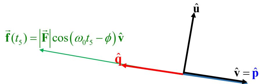
**The vector  $\vec{f}(t)$  does not change its direction and its tip moves along a straight line**
