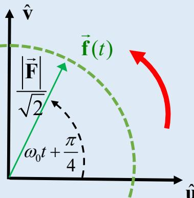
The vector  $\vec{f}(t)$  maintains a constant modulus and its tip moves along a circle with angular velocity  $\omega_0$
