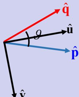
The vector  $\vec{f}(t)$  lies in the polarization plane  $(\hat{\mathbf{p}}, \hat{\mathbf{q}})$  (which is coincident with the plane  $(\hat{\mathbf{u}}, \hat{\mathbf{v}})$ ), and it changes in general both its amplitude and its direction as the time elapses.
