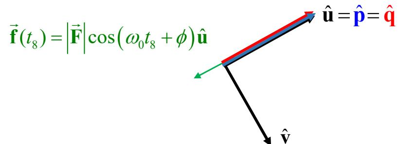
The vector  $\vec{f}(t)$  does not change its direction and its tip moves along a straight line
