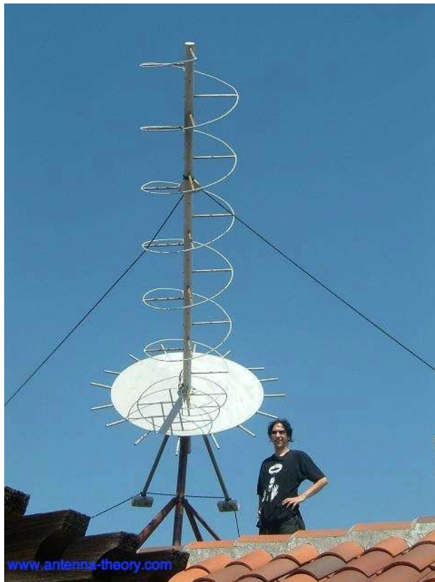
Helix or helical antenna
