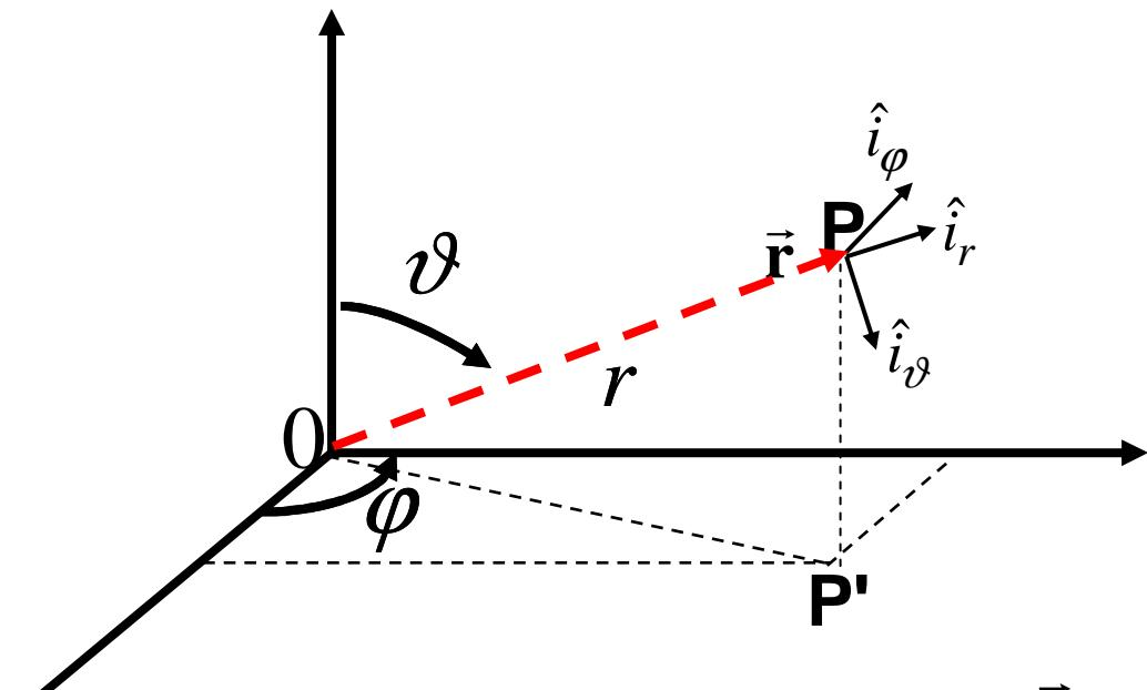
$$\begin{aligned}\hat{i}_\phi &= \hat{i}_r \times \hat{i}_\vartheta \\ \hat{i}_\vartheta &= \hat{i}_\phi \times \hat{i}_r \\ \hat{i}_r &= \hat{i}_\vartheta \times \hat{i}_\phi\end{aligned}$$
