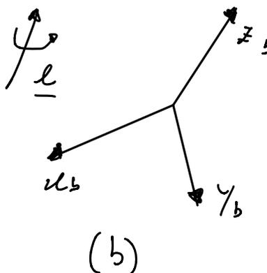
$$C_a^b = \cos(-\theta) I_3 + [1 - \cos(-\theta)] \underline{e} \underline{e}^T + \sin(-\theta) A(\underline{e})$$
