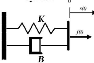
*B*, viscous friction coeff. of the damper  $f(t) + f_e(t) + f_d(t) = 0$  $f_d(t) = -B\dot{s}(t)$ x(t) = s(t)
