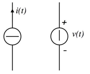
▲ An ideal current (voltage) source provide a current that passes through it (a voltage at its terminals) that is independent of the network in which it is inserted.
