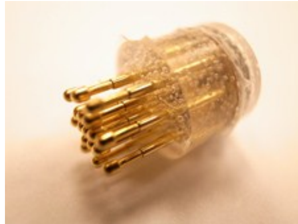
Spring-loaded Pins (NCTU)
