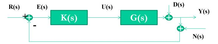
The transfer function  $D(s) \to Y(s)$  o (E(s)) is the same as the transfer function  $R(s) \to E(s)$  (except for the sign for E(s) = -S(s)D(s)).
