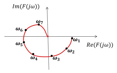
F(s) is represented in the polar plane as a function of  $j\omega$ assuming  $\omega$  moving from 0 to  $+\infty$
