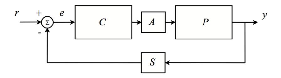
A closed-loop feedback control system uses a sensor S to continuously «feed back» a measurement of the actual output of the system.
