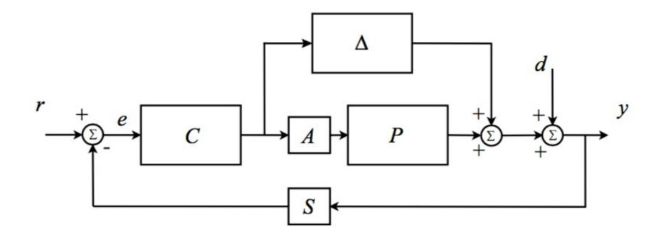
Assuming that *S*=1 (excellent quality of sensor/transducer, which is not affected by noise),
