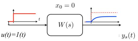
▲ The "decaying" exponential functions determine *the transient* part of the response while the constant term is the *steady-state* value.
