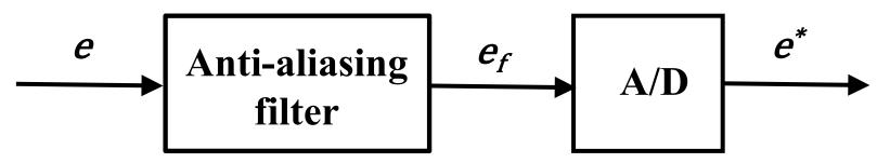
In this way the spectrum of the signal to be sampled doesn't have significant components for  $\omega > \omega_f$
