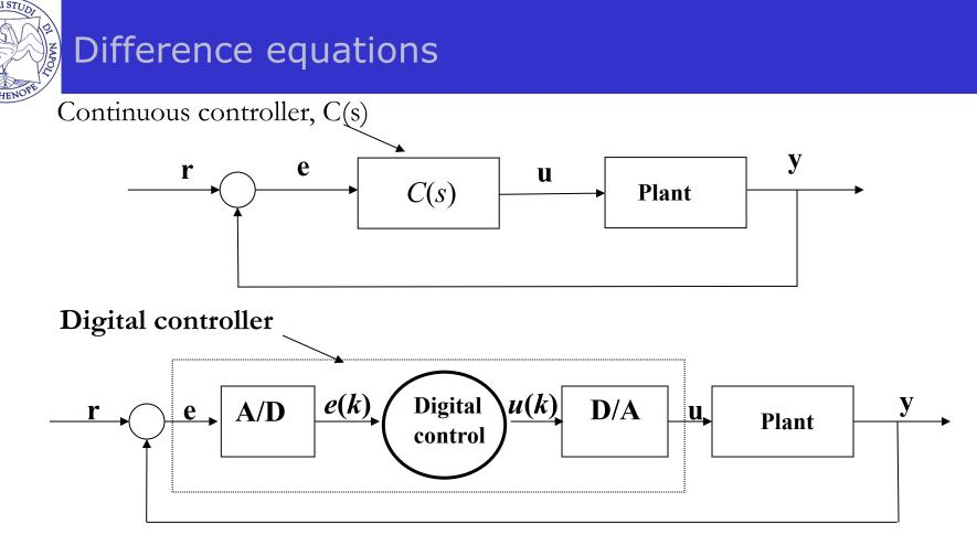
Assume that A/D takes sample of continuous signal e(t) at discrete times and passes them to the controller/computer:  $\hat{e}(kT) = e(kT) = e(k)$ .
