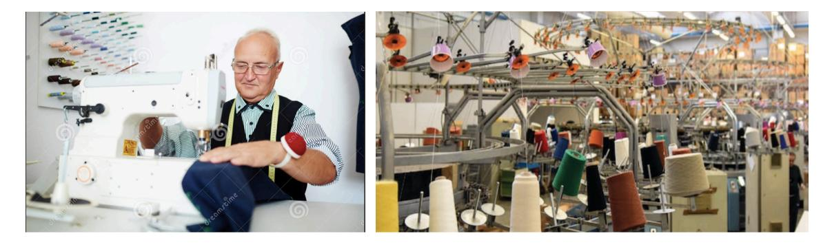
a skilled worker (tailor) will use a general purpose machine (sewing machine) to run off a small batch **production-line manufacture**, a specialised machine will be programmed and used
