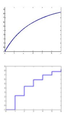
**analog signals,** if the amplitude can vary continuously in an interval of  $\mathbb{R}$
