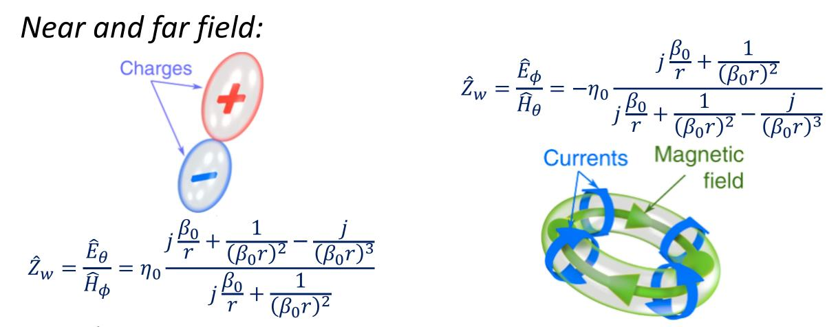
$\hat{Z}_w$  is termed as wave impedance ("intrinsic impedance" in the far field case).
