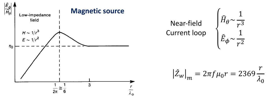
Hence, in the near field, the current loop is termed as **low impedance source** since its wave impedance is lower than the intrinsic one.
