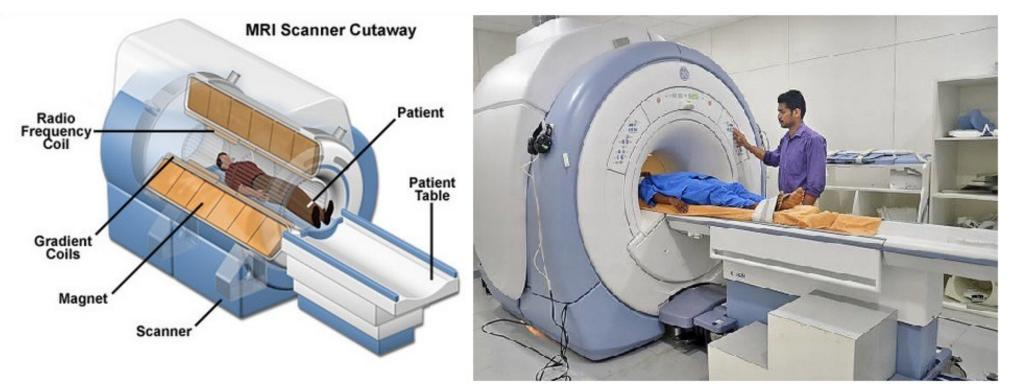
A static magnetic field (1.5 T or 3 T) is used in Magnetic Resonance Imaging
