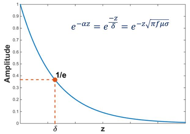
The penetration depth  $\delta$  is defined as the depth where the power density is just 1/e (about 37%) of the surface value.
