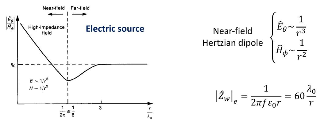
Hence, in the near field, the electric dipole is termed as **high impedance source** since its wave impedance is larger than the intrinsic one.
