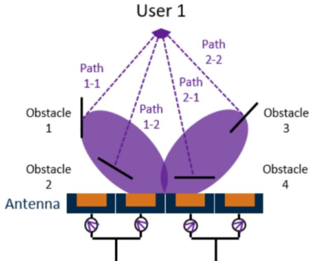
Four Radiating Elements at a common frequency with  $45^\circ$  the other with  $-45^\circ$  phase shift supporting MIMO for increasing SNR and channel capacity
