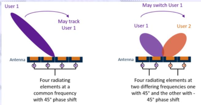
The direction a signal is sent in is calculated dynamically by the base station as the endpoint moves, effectively tracking the user.
