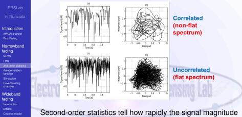
Frequency domain Overcome wideband fading Second-order statistics tell how rapidly the signal magnitude changes between different levels. This info is commonly specified in terms of spectrum of the signal.
