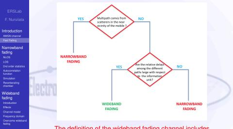
The definition of the wideband fading channel includes characteristics of both the signal and the channel.
