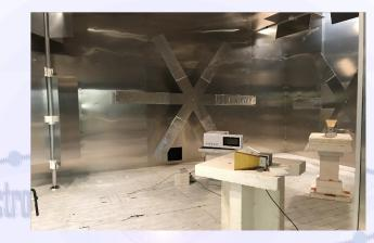
A microwave electrically-large metallic chamber where the field is made random and on the average uniform and isotropic by means of a proper stirring.
