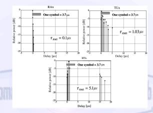
Example of measured GSM PDPs profiles related to macrocells that refer to Rural Area (RA), Typical Urban (TU) and Hilly Terrain (HT).
