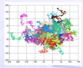
The received signal consists of a multipath random (Rayleigh-distributed) component plus a coherent LOS component.
