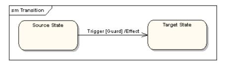
"Trigger" is the cause of the transition, which could be a signal, an event, a change in some condition, or the passage of time.
