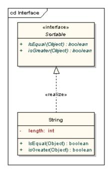
Interfaces may be drawn in a similar style to a class, with operations specified, as shown below. They may also be drawn as a circle with no explicit operations detailed. When drawn as a circle, realization links to the circle form of notation are drawn without target arrows.
