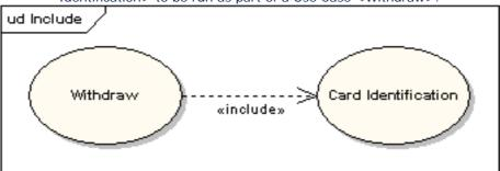
Use Cases may be included by one or more Use Case, helping to reduce the level of duplication of functionality by factoring out common behavior into Use Cases that are re-used many times.
