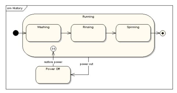
In this state machine, when a washing machine is running it will progress from Washing through Rinsing to Spinning. If there is a power cut, the washing machine will stop running and will go to the Power Off state. Then when the power is restored, the Runnin state is entered at the History State symbol meaning that it should resume where it last left-off.
