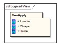
Packages are represented in UML 2.0 as folders and contain the elements that share a namespace; all elements within a package must have a unique identifier. The Package must show the Package name and can optionally show the elements within the Packag in extra compartments.
