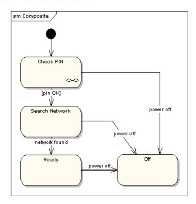
The notation in the above version indicates that the details of the Check PIN sub-machine are shown in a separate diagram.
