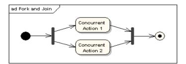
A join is different from a merge in that the join synchronises two inflows and produces a single outflow. The outflow from a join cannot execute until all inflows have been received. A merge passes any control flows straight through it. If two or more inflows ar received by a merge symbol, the action pointed to by its outflow is executed two or more times.
