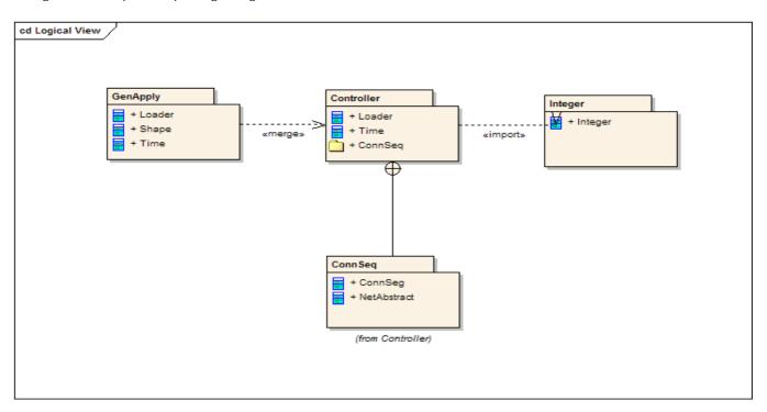
Elements contained in a Package share the same namespace, this sharing of namespace requires the elements contained in a specific namespace to have unique names.
