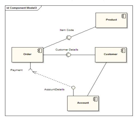
Components are similar in practice to package diagrams as the define boundaries and are used to group elements into logical structures. The difference between Package Diagrams and Component diagrams is that Component Diagrams offer a more semantically rich grouping mechanism. With Component Diagrams all of the model elements are private whereas Package diagrams only display public items.
