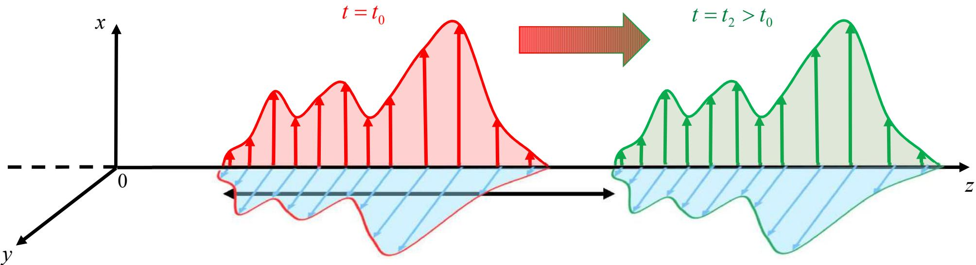
The electromagnetic perturbation **propagates** without deformation and with constant speed  $c$  along the positive sense of the  $z$ -axis
