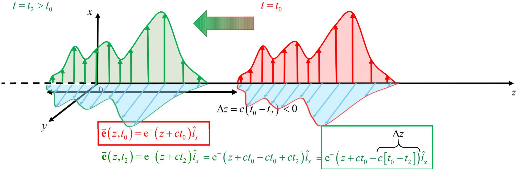
The electromagnetic perturbation **propagates** without deformation and with constant speed **c** along the negative sense of the z-axis
