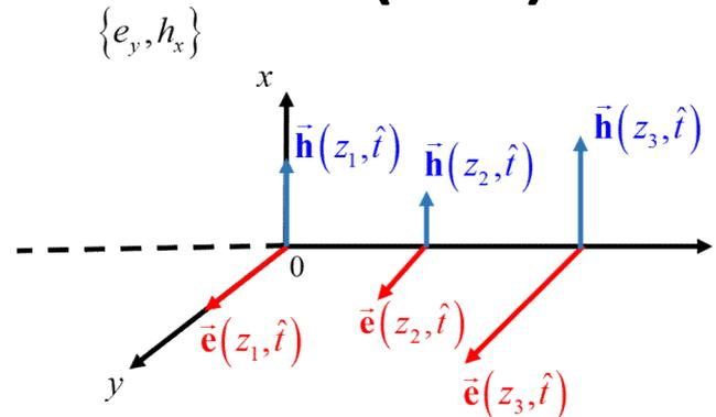
$$\begin{cases} \frac{\partial e_x}{\partial z} = -\mu \frac{\partial h_y}{\partial t} \\ \frac{\partial h_y}{\partial z} = -\epsilon \frac{\partial e_x}{\partial t} \end{cases} \quad \frac{\partial^2 e_x}{\partial z^2} = \mu\epsilon \frac{\partial^2 e_x}{\partial t^2} \quad \frac{\partial^2 e_x(z,t)}{\partial z^2} - \frac{1}{c^2} \frac{\partial^2 e_x(z,t)}{\partial t^2} = 0$$
