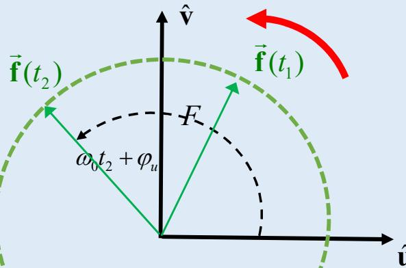
$$(|F_u| = |F_v| = F) \quad \text{and} \quad \left( \varphi_v - \varphi_u = \frac{\pi}{2} \right)$$
