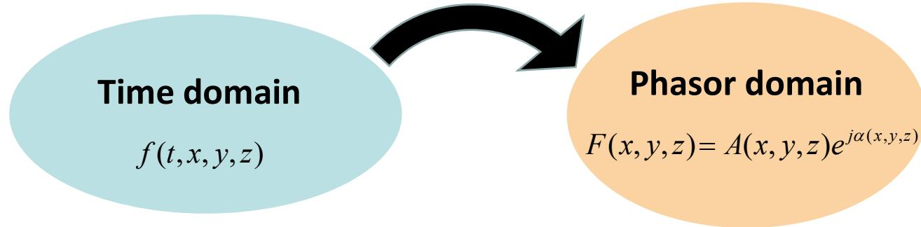
$$f(t, x, y, z) = A(x, y, z) \cos(\omega_0 t + \alpha(x, y, z))$$
