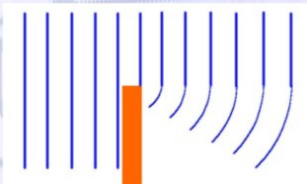
Even if a region is shadowed by an obstruction, diffraction around the object's edges produces waves that propagate into the shadowed region.
