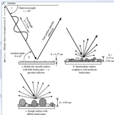
The reflected wave is scattered by a large number of scattering points on the surface. This process results in a broadening of the scattered energy.
