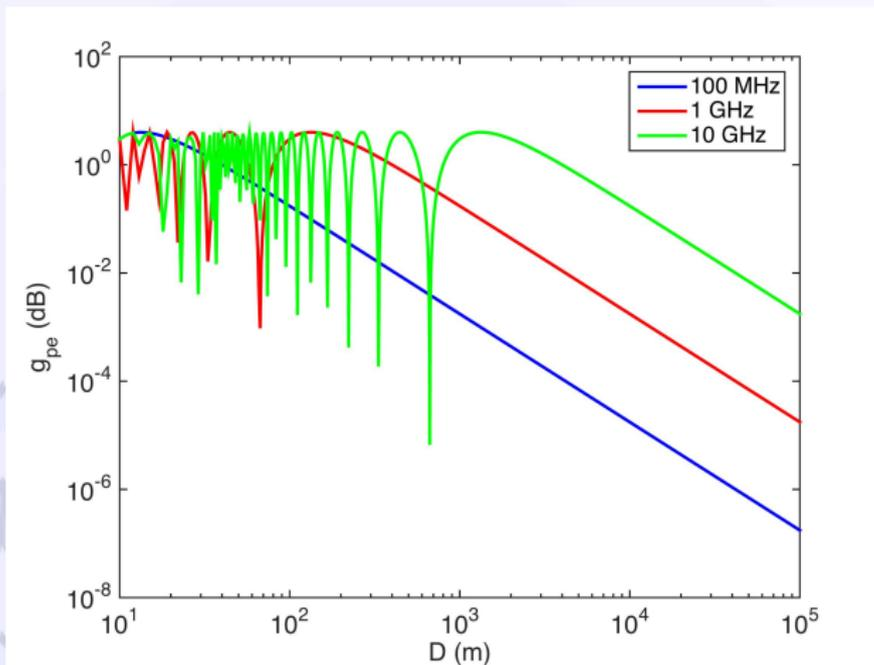
The effects of constructive/destructive interference between the LOS and reflected waves depend on  $h_1, h_2, D, \lambda$ .
